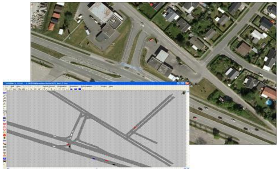
Fig. 1.1. Microsimulation of traffic is a representation of real road networks and traffic flow in a detailed model.
